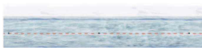
Construction: 50-metre spacing between auger test holes along road centre line
