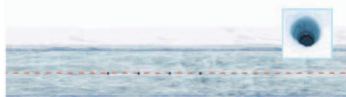
Pre-construction: 10-metre spacing between auger test holes along centre line
