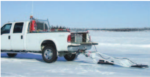
Dual channel GPR ice profiling equipment (being pulled behind a truck) measuring ice thickness and water depth in a single pass
