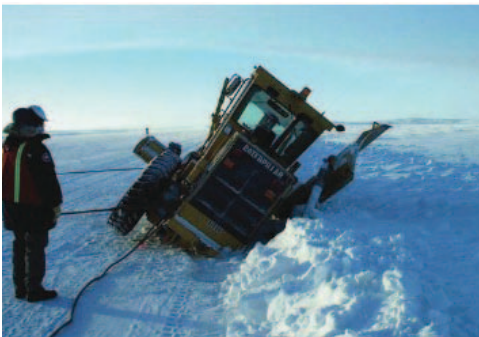
Grader partially broken through thin ice beneath a snowbank
