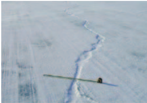
Longitudinal ice contraction crack
